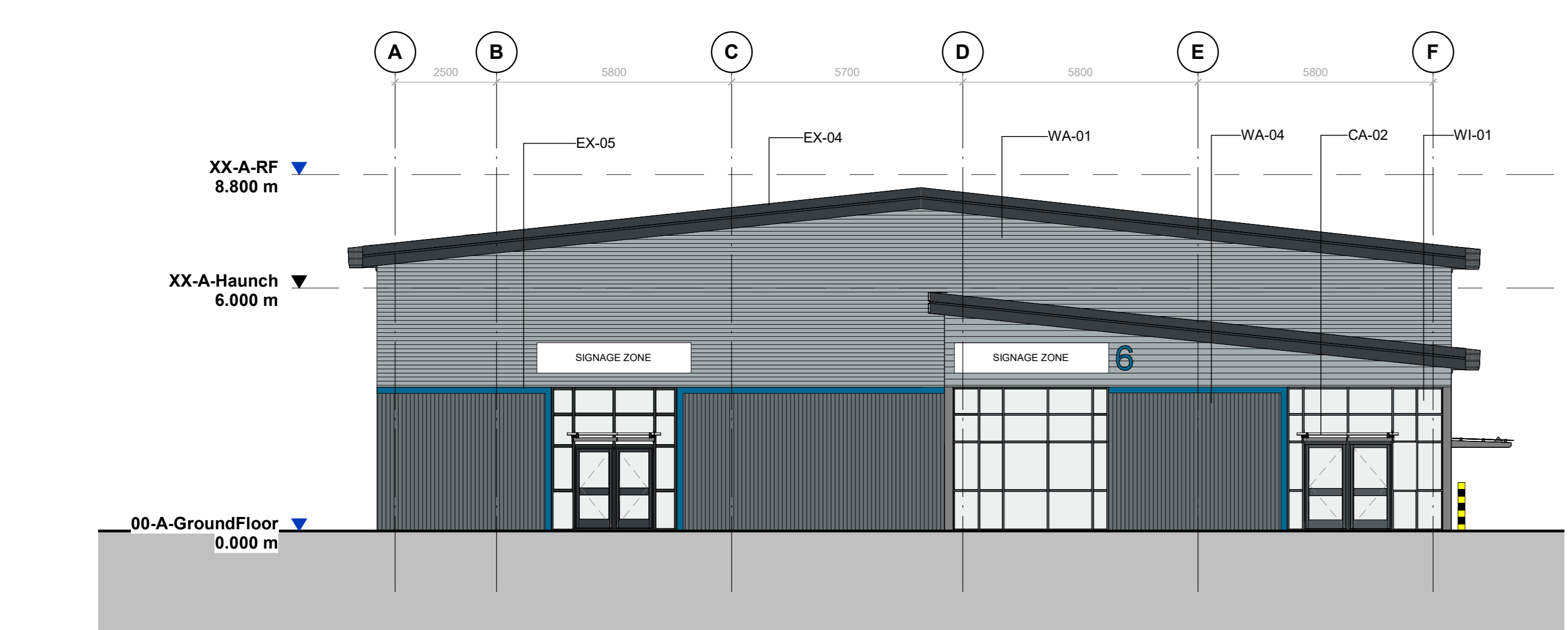
Unit 1-6 East Elevation 1 : 100
